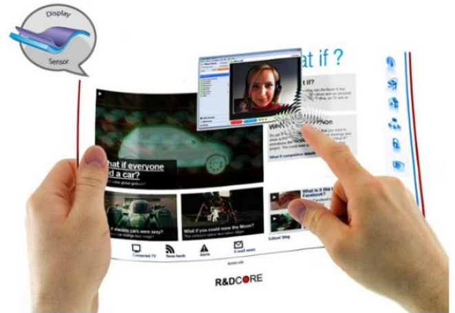
Fig. 1 - Touchscreen placed behind a flexible display
